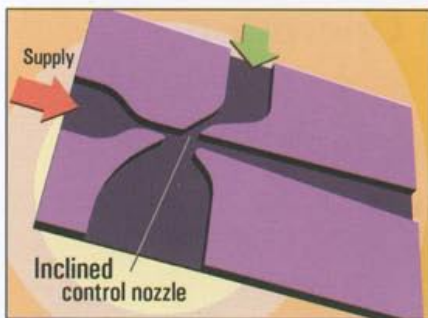
Figure 5 Improvement of efficiency of the control action may be obtained by inclining the control nozzle against the supply flow from the main nozzle
