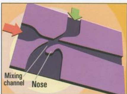
Figure 7 Important development step in the history of pressure-driven microfluidic valves was the introduction of the „nose” in the inclined control jet devices, achieving the double purpose preventing „short-circuiting” flow into collector entrance and enhancing the control effect by jet pumping
